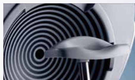
Placido disk - Measurement of corneal curvature radius
