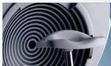
Placido disk - Measurement of corneal curvature radius
